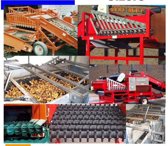
The **Mayo Roller Sizers** are available as portable units or installed in sorting and packing lines. They come in a variety of sizes and configurations. Each is designed for the specific application required. Options include cross and discharge conveyors.
