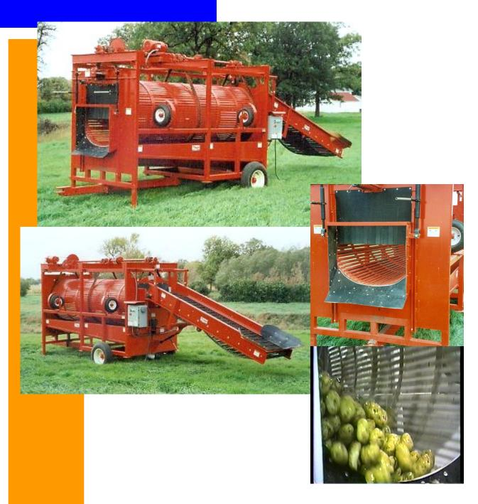
The **Mayo Barrel Washer** will wash chip and process potatoes with less water and allow better sorting. Portability and variable speed control make it an effective machine in your operation. Options include discharge pump and water recirculator.
