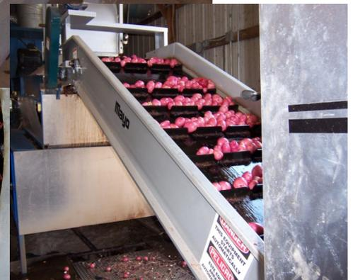
The **Mayo Washer Polisher** utilizes rotary brushes combined with speed control and elevation control to clean potatoes. Options include presoak Flume Tank and Discharge Conveyors
