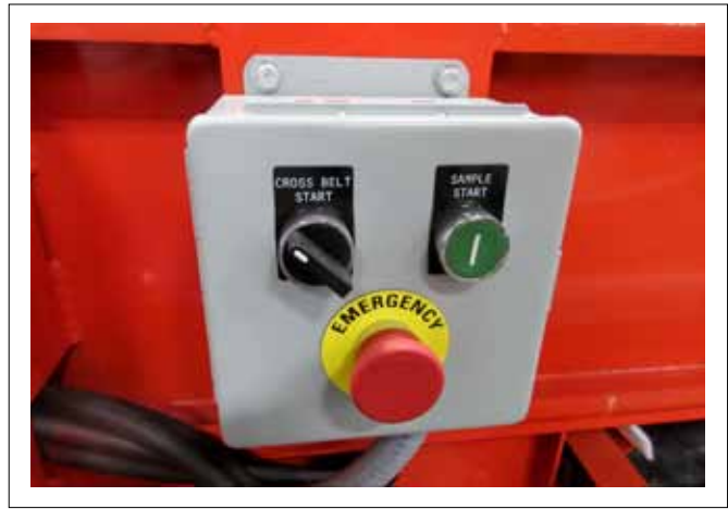
FIG. 18 CROSS CONVEYOR CONTROLS
