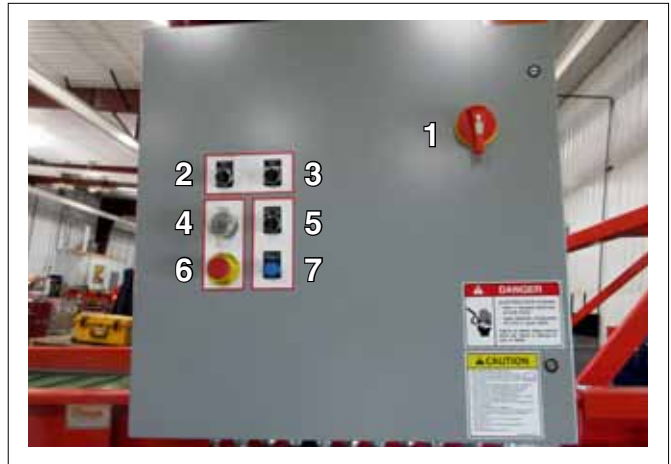
FIG. 4 CONVEYOR CONTROLS (TYPICAL)
