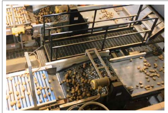
FIG. 11 SIZING SYSTEM (TYPICAL)
