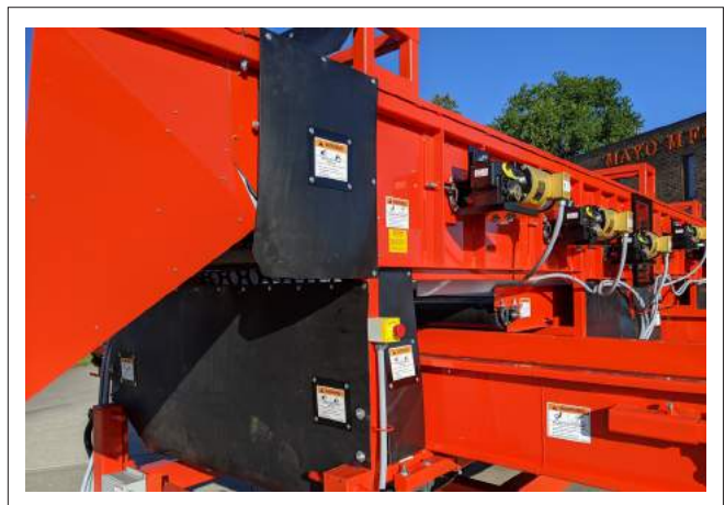
FIG. 14 EMERGENCY STOP - FRAME
