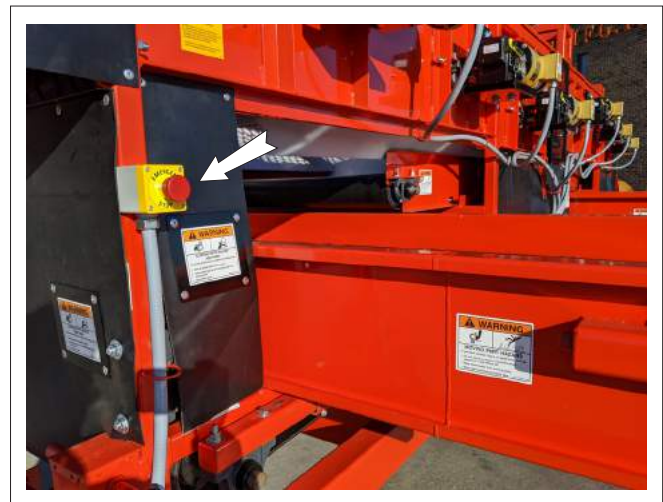
FIG. 5 EMERGENCY STOP - FRAME
