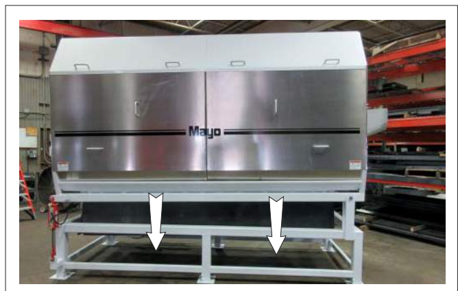
FIG. 22 WATER CONTAINMENT AREA
