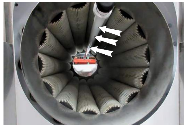
Water Holes (Typical)
