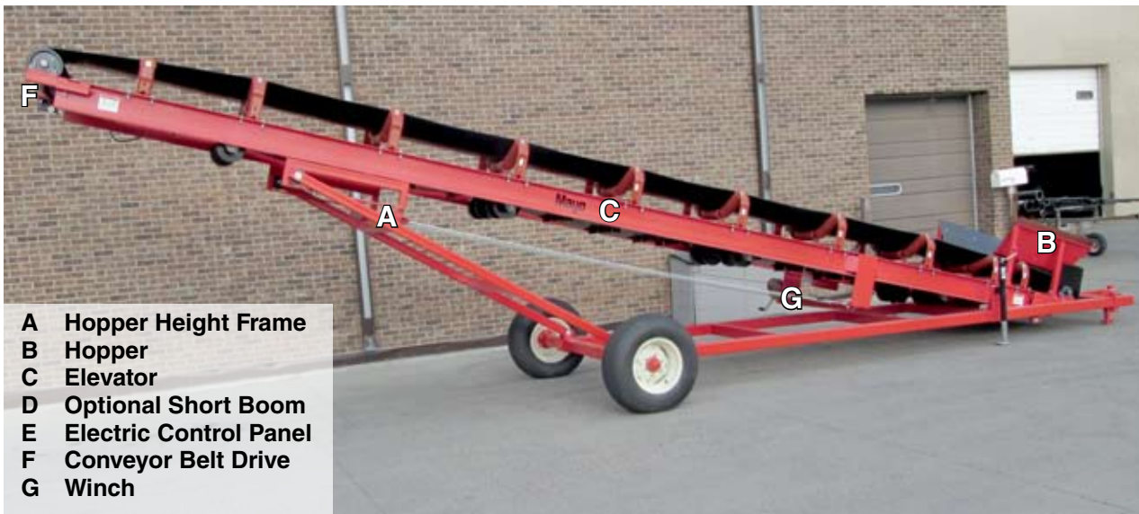
FIG. 1 MACHINE COMPONENTS
