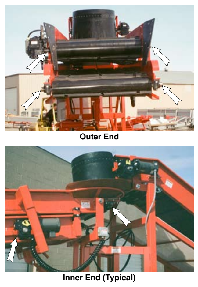
FIG. 35 BOOM CONVEYOR SHAFTS
