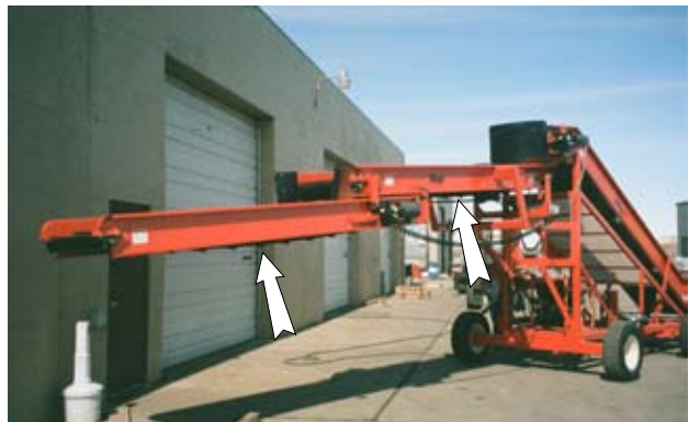
Boom Conveyor Sag (Typical)
