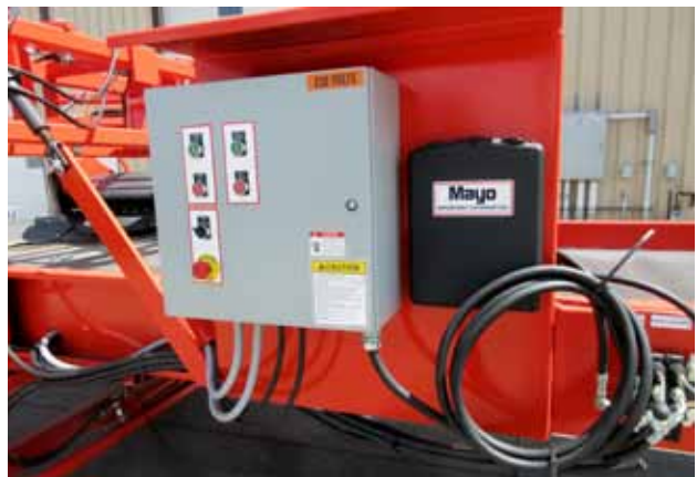
Conveyor with Stinger and Hydraulic Power Pack
