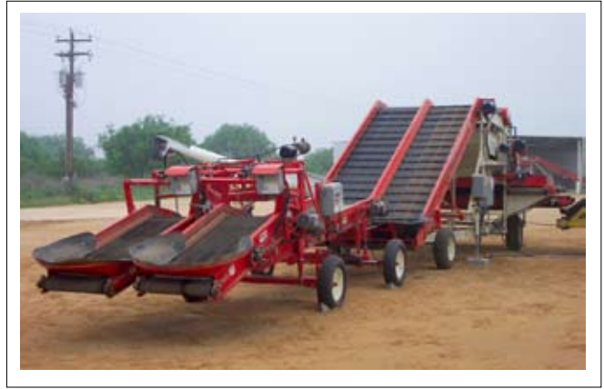
FIG. 14 UNLOADING CONVEYOR (TYPICAL)
