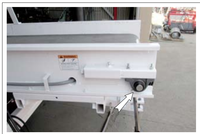
FIG. 24 CONVEYOR SHAFTS (TYPICAL)
