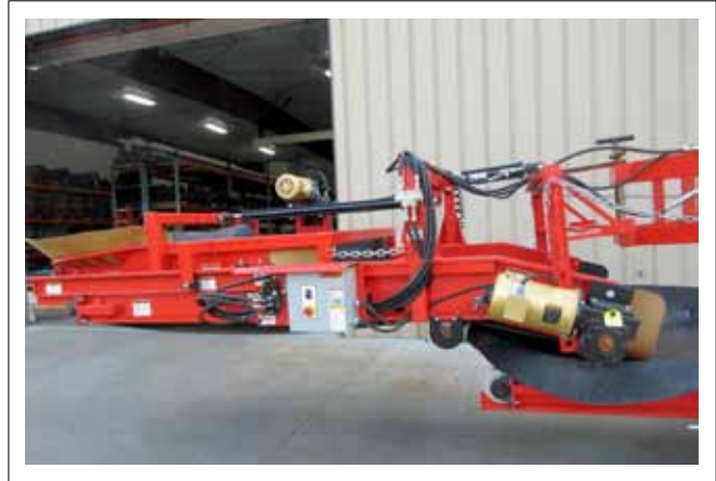
FIG. 9 ELECTRIC & HYDRAULIC LINES (TYPICAL)
