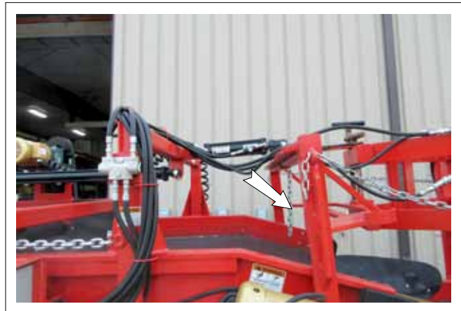
FIG. 22 SIDE SWING ANCHOR CHAIN
